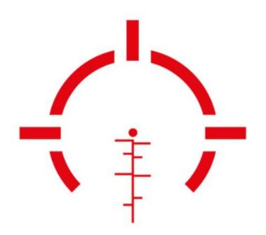
Our prism optics are equipped with an advanced ballistic reticle that enables precise shot placement over various distances up to 500 metres. Thanks to special markings and lines in the reticle for .223 Rem and .308 Win calibres, corrections can be made quickly and accurately for a safe shot without losing the aiming line. This precisely calibrated reticle offers a decisive advantage for hunting or sport shooting.
